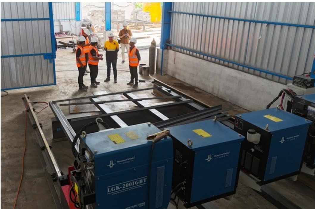
Photo 6: Inspecting Automatic Plasma and Laser cutting unit. Steel cutting design is completed in the workshop engineering office and downloaded to the cutting unit for execution.
