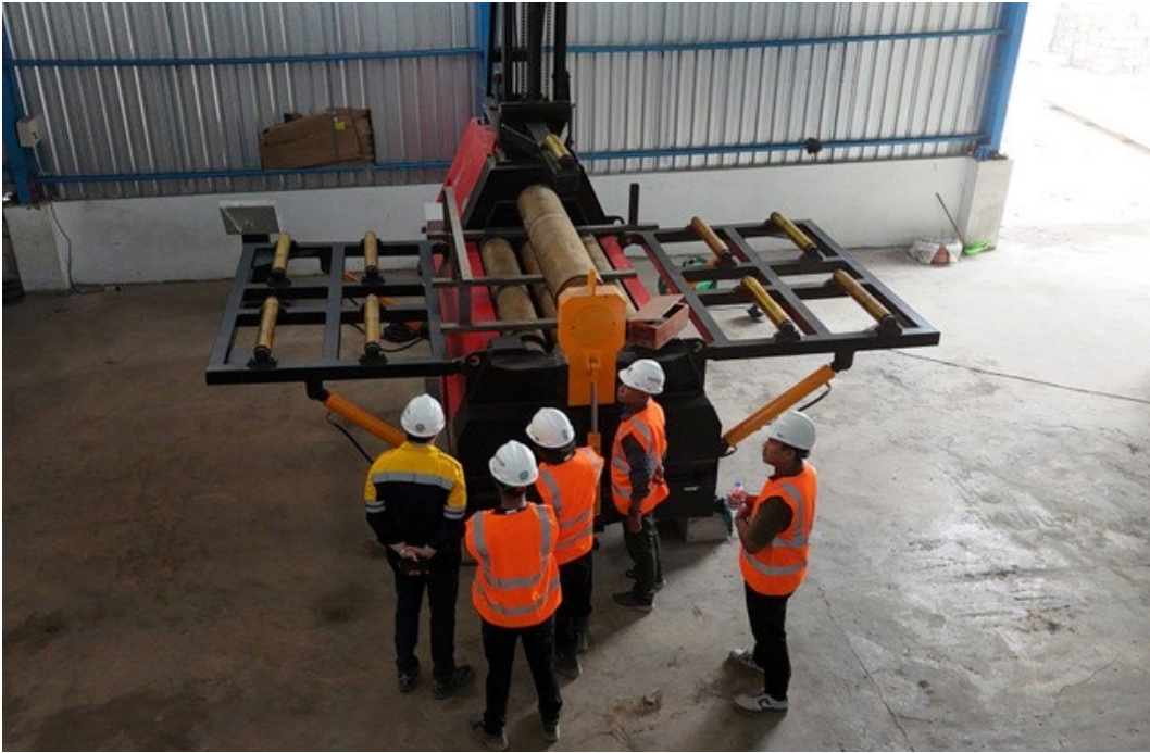
Photo 6: Inspecting Automatic Plasma and Laser cutting unit. Steel cutting design is completed in the workshop engineering office and downloaded to the cutting unit for execution.
