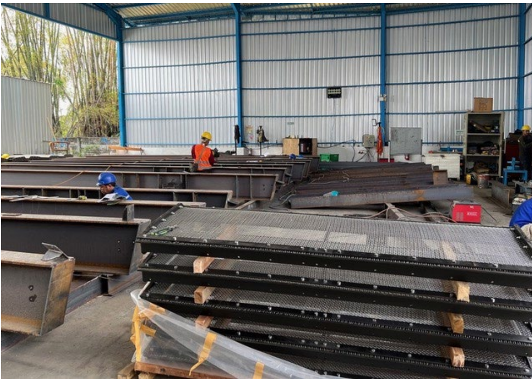
Photo 4: Examples of large structural steel fabricated pieces awaiting protective coating.
