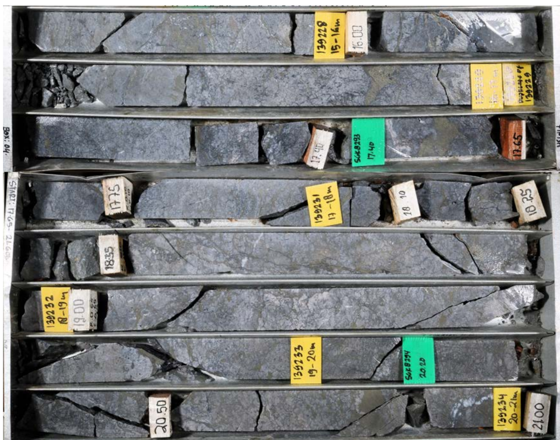
Figure 2: (Top) High grade chalcocite – covellite mineralisation in BKM32230-01. The weighted average grade for the interval 114.5 – 117.5 metres is 1.98% Cu. (Bottom) High grade chalcocite – covellite mineralisation in BKM31720-01. The weighted average grade for the interval 16 – 22 metres is 2.73% Cu
