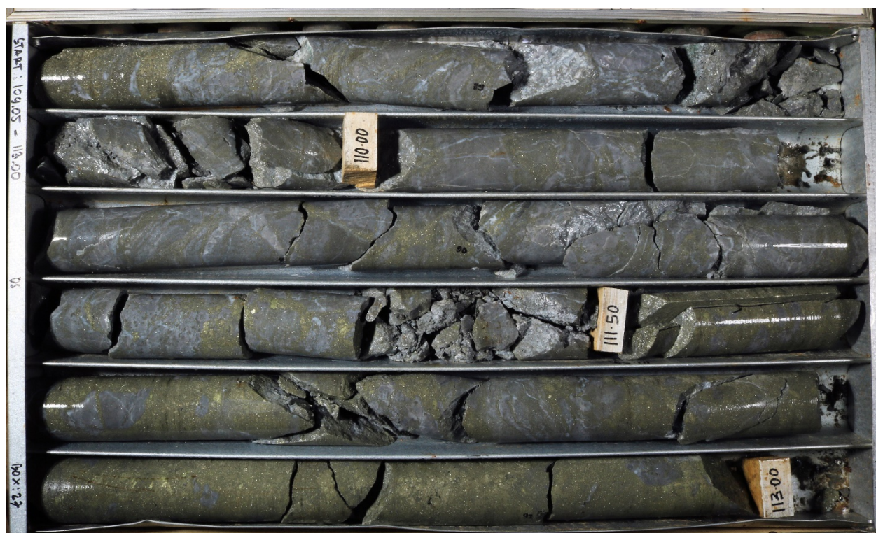
Figure 4: Semi-massive sulphides with strong chalcopyrite mineralisation in BKZ33650-02.
