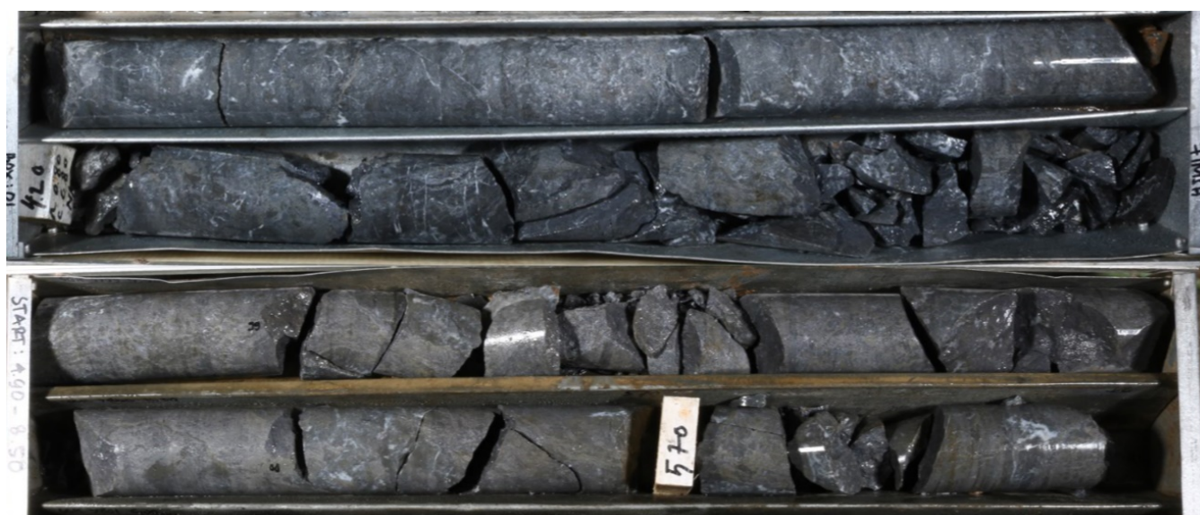
Figure 2: Semi-massive Sphalerite (Zn sulphide) and Galena (Pb sulphide) mineralisation in BKZ33750-02. The weighted average grade for the interval 4 – 6m (2m interval) is 17.1% Zn, 8.7% Pb and 83g/t Ag
