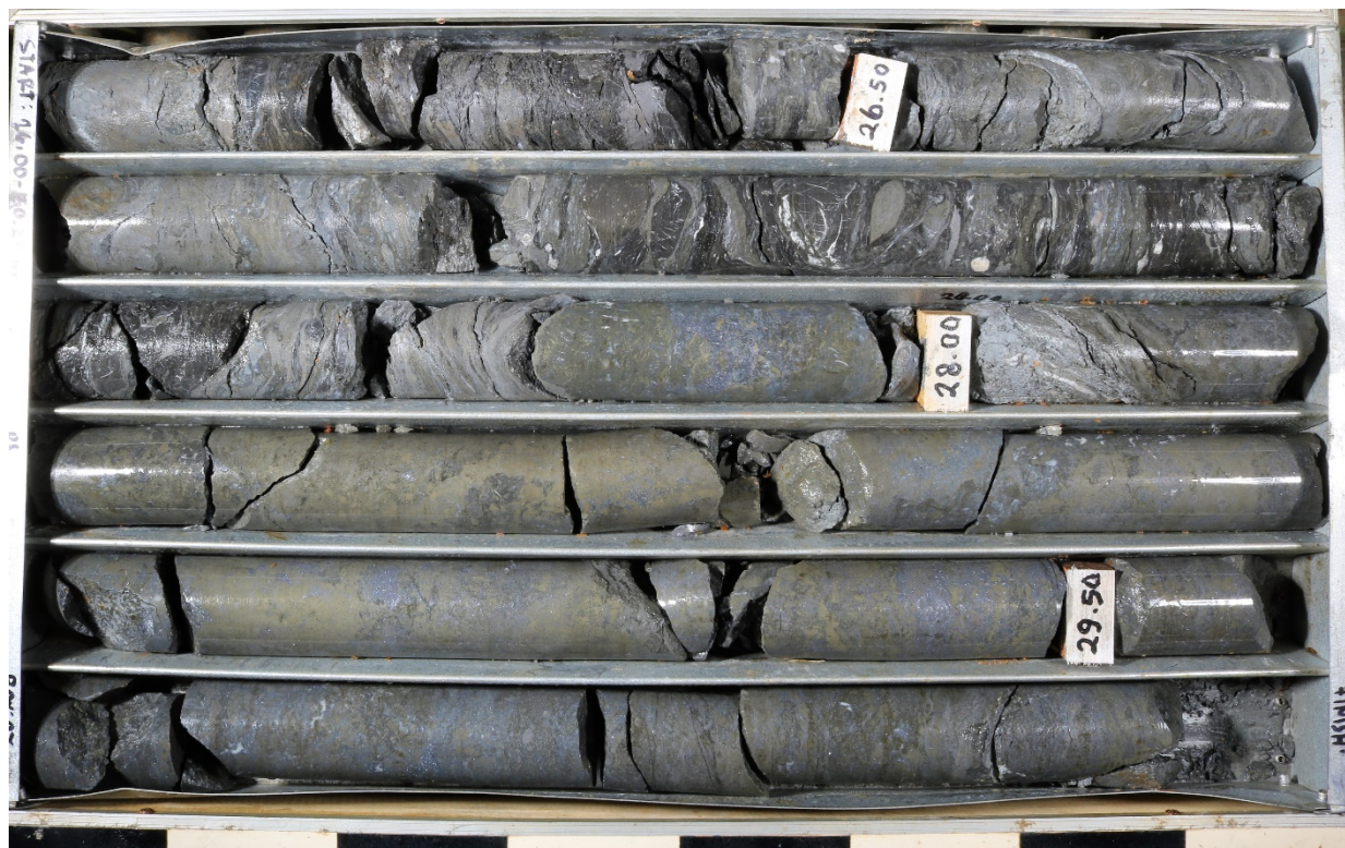
Figure 3: Massive sulphides with strong galena mineralisation in BKZ33750-03, assays pending.
