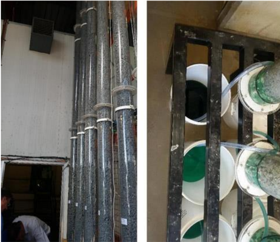
Figure 1: (Left) BKM 6-metre Leach Columns at CORE Laboratories (Right) PLS (Pregnant Liquor Solution) from Leach Column Discharge (Showing copper dissolution via characteristic green colour)
