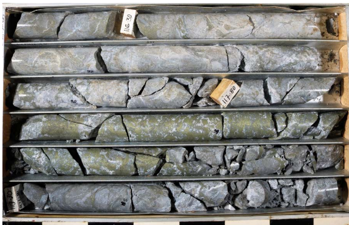
Figure 4: High grade copper mineralisation in BKZ33600-03. The interval 118m - 119m (1m interval) is 11.80% Cu and 19.5g/t Ag.
