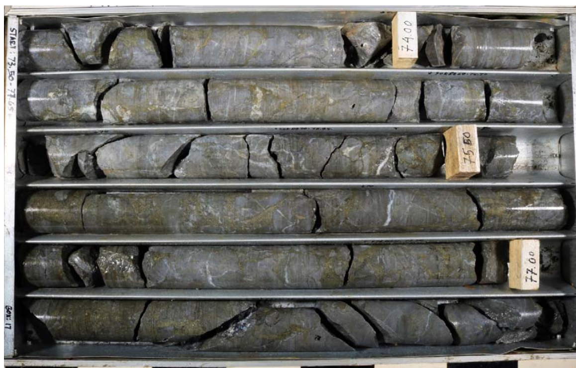
Figure 3: Feeder zone mineralisation in BKZ33600-02. The weighted average grade for the interval 74m - 78m (4m interval) is 2.80% Cu and 23.2g/t Ag.
