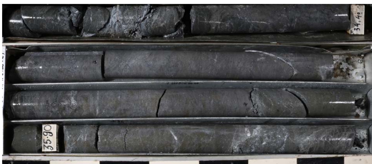
Figure 2: Semi-massive Sphalerite (Zn sulphide) and Galena (Pb sulphide) mineralisation in BKZ33600-01. The weighted average grade for the interval 34m - 36m (2m interval) is 15.6% Zn, 7.2% Pb and 102.1g/t Ag
