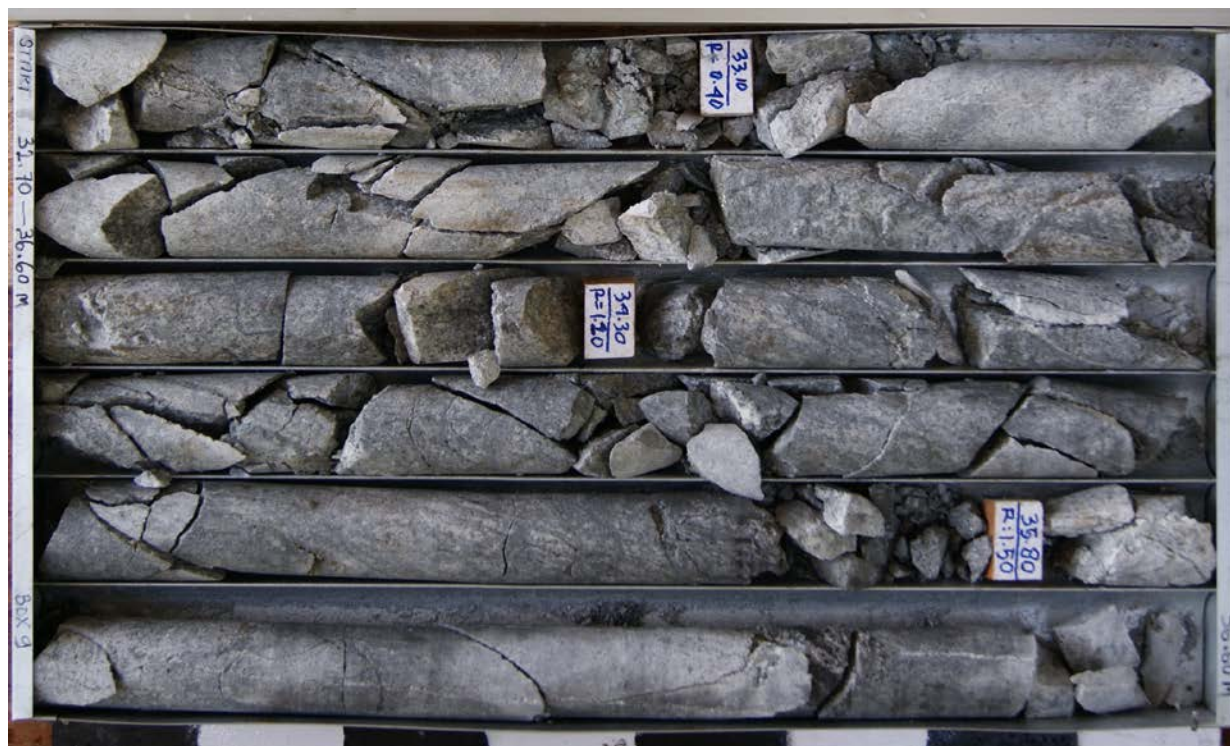
Figure 3: Drill core from Beutong East Porphyry showing strong stockwork with secondary sulphide mineralisation. Drill hole BEU0800-01, interval 32.5 – 36.8m (4.3m interval) assayed 1.67% Cu and 0.18g/t Au
