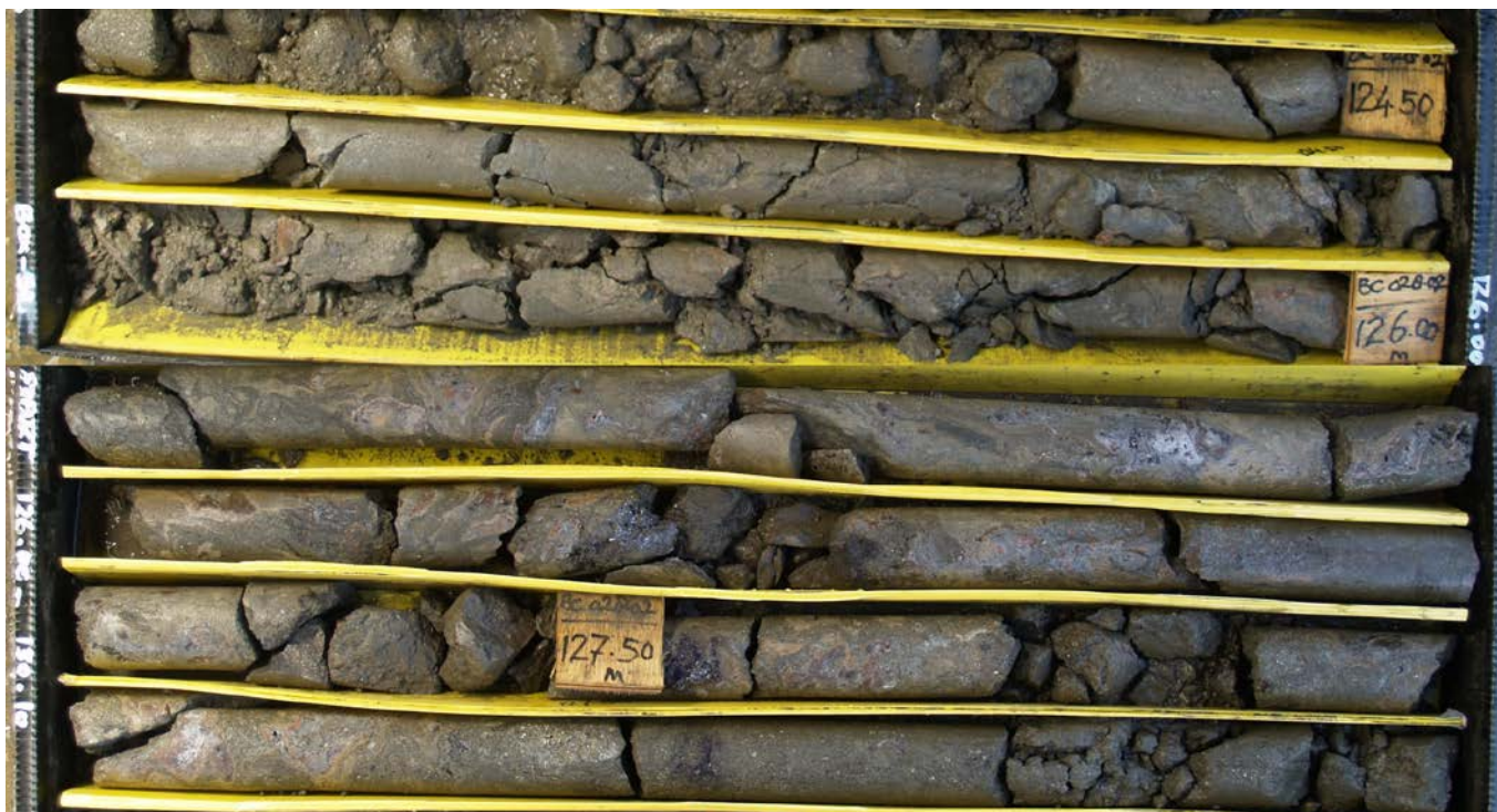
Figure 5: Drill core from Beutong's BC28 Zone, showing a Garnet skarn with high grade polymetallic mineralisation. Drill hole BC028-02, interval 125 – 130.5m (5.5m interval) assayed 1.7% Cu, 0.37g/t Au, 10.9% Zn and 3.32% Pb
