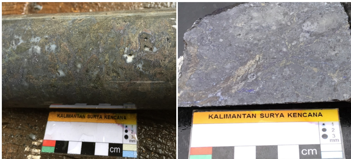
Figure 2: (Left) massive sulphide mineralisation in BKZ33750-05 (32.5m depth), comprising pyrite-sphalerite-galena. (Right) Bornite in mm-scale veins and as disseminated grains in BKZ33750-03 (50.5m depth).
