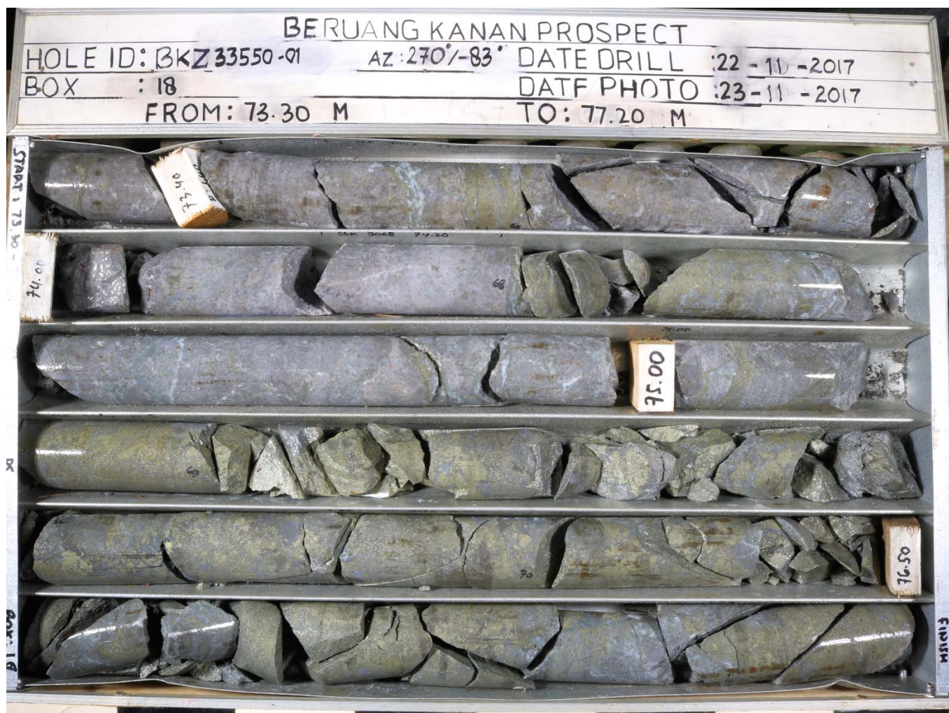
Figure 3: High grade copper mineralisation in BKZ33550-01. The interval 74m - 77m (3m interval) is 3.0% Cu and 13g/t Ag
