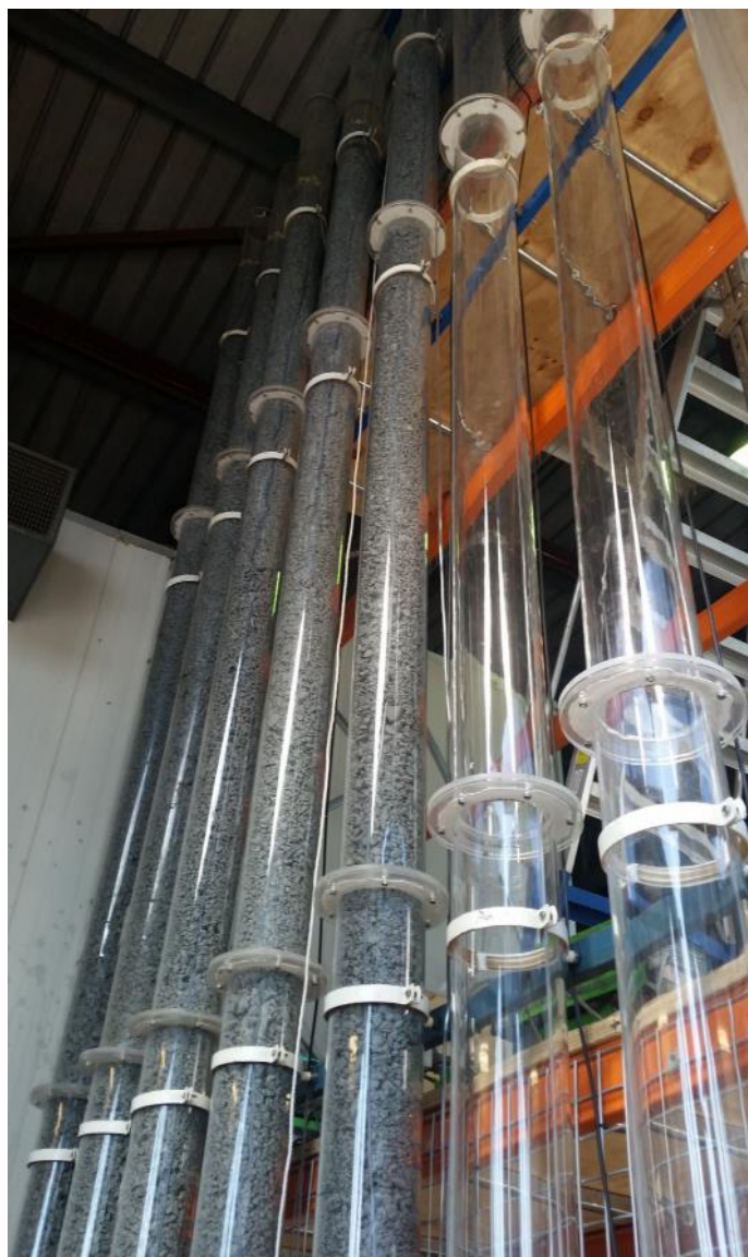
Figure 2: Long Columns being loaded at CORE Laboratory
