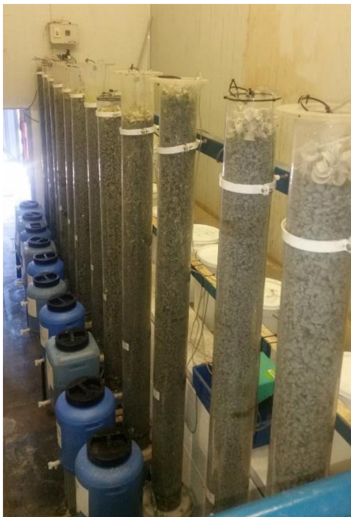
Figure 1: Short Columns loaded and under leach at CORE Laboratory
