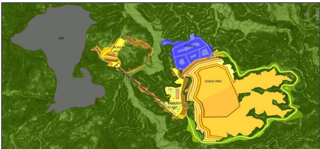
Figure 2 – Mine and Process Area Layout
