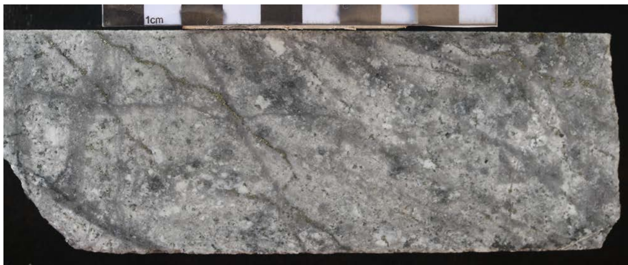
Figure 2: High grade copper mineralisation intersected at end of drill hole BEU1350-02, with the final 4-metres assaying 0.82% Cu.
