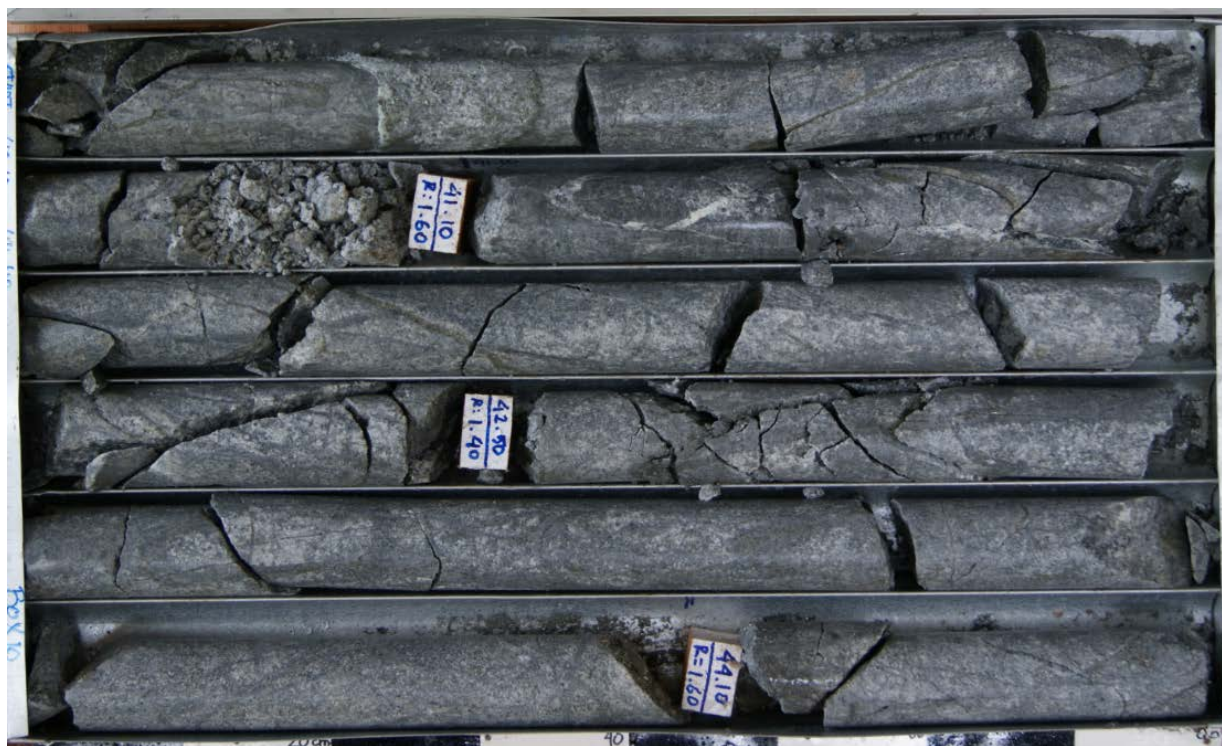
Figure 3: Drill core from Beutong East Porphyry showing strong stockwork with secondary sulphide mineralisation. Drill hole BEU0800-02, interval 41.2 – 45.6m (4.4m interval) assayed 2.0% Cu and 0.19g/t Au
