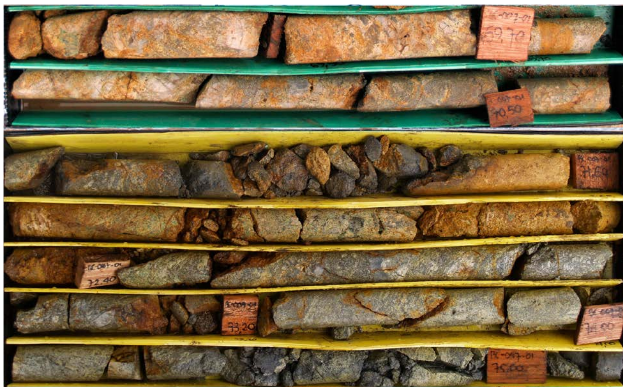
Figure 4: Drill core from Beutong Skarn showing strong copper oxide mineralisation (malachite, Azurite). Drill hole BC007-01, interval 69 – 75m (6.0m interval) assayed 3.84% Cu, 1.58g/t Au and 0.87% Zn
