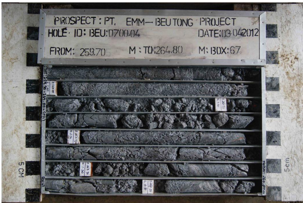
Figure 21: Core showing significant clay alteration and partial core loss.
