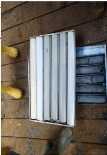
Drill cores should be covered by halve PVC pipes before being covered by plywood lids
