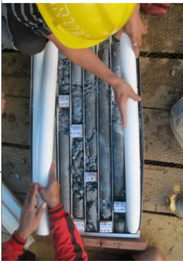
Drill cores should be covered by halve PVC pipes before being covered by plywood lids
