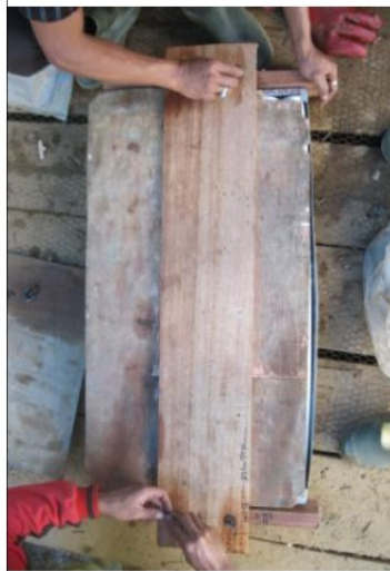
Drill cores should be covered by halve PVC pipes before being covered by plywood lids
