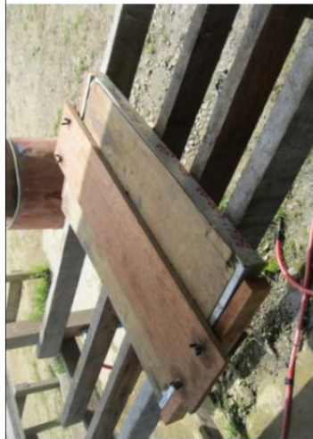
Drill cores should be covered by halve PVC pipes before being covered by plywood lids
