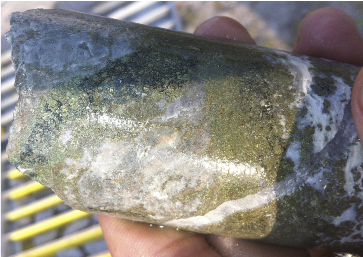
Plate 3: BK029, 90m – Covellite disease of massive pyrite.
