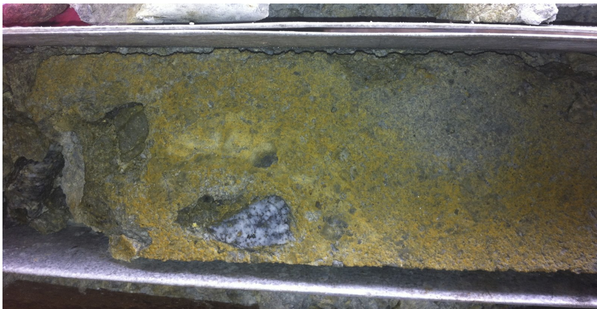
Plate 7: BK057, 19m – silica-covellite vein fragment within fault gouge material.
