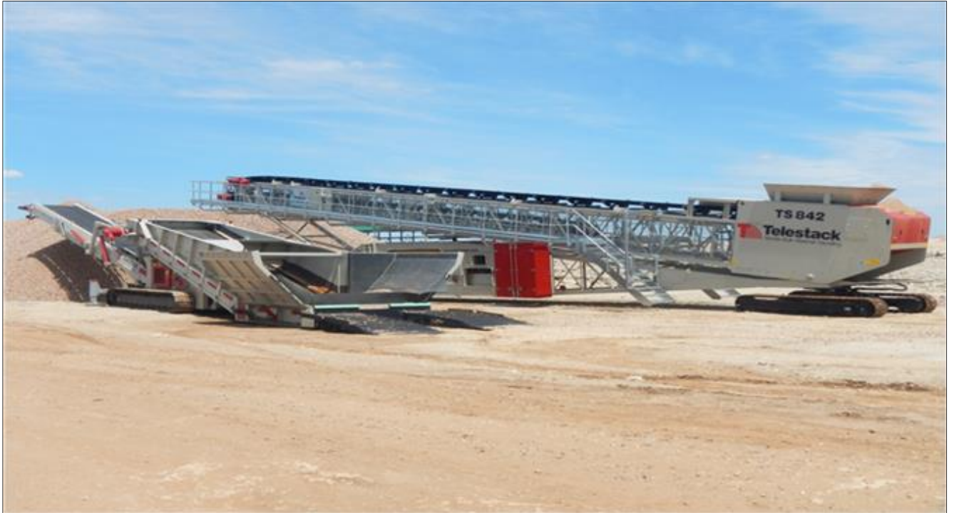
Figure 17-5 Stacker and dump hopper (ready for relocation)
