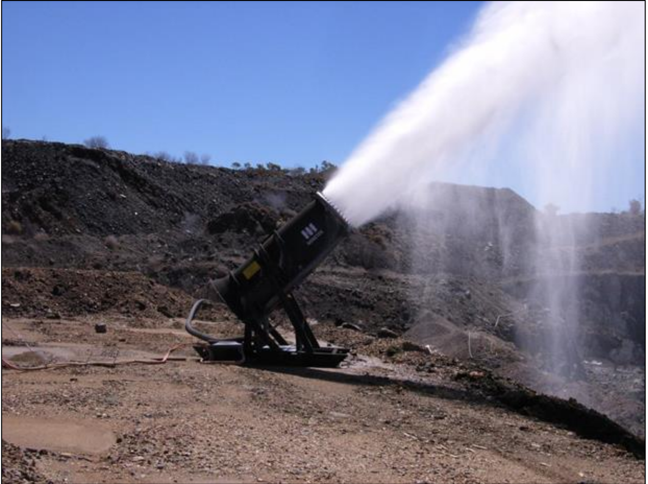
Figure 17-12 Water cannon in operation evaporating water.
