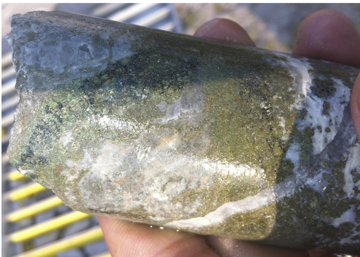
Plate 3: BK029, 90m – Covellite disease of massive pyrite.
