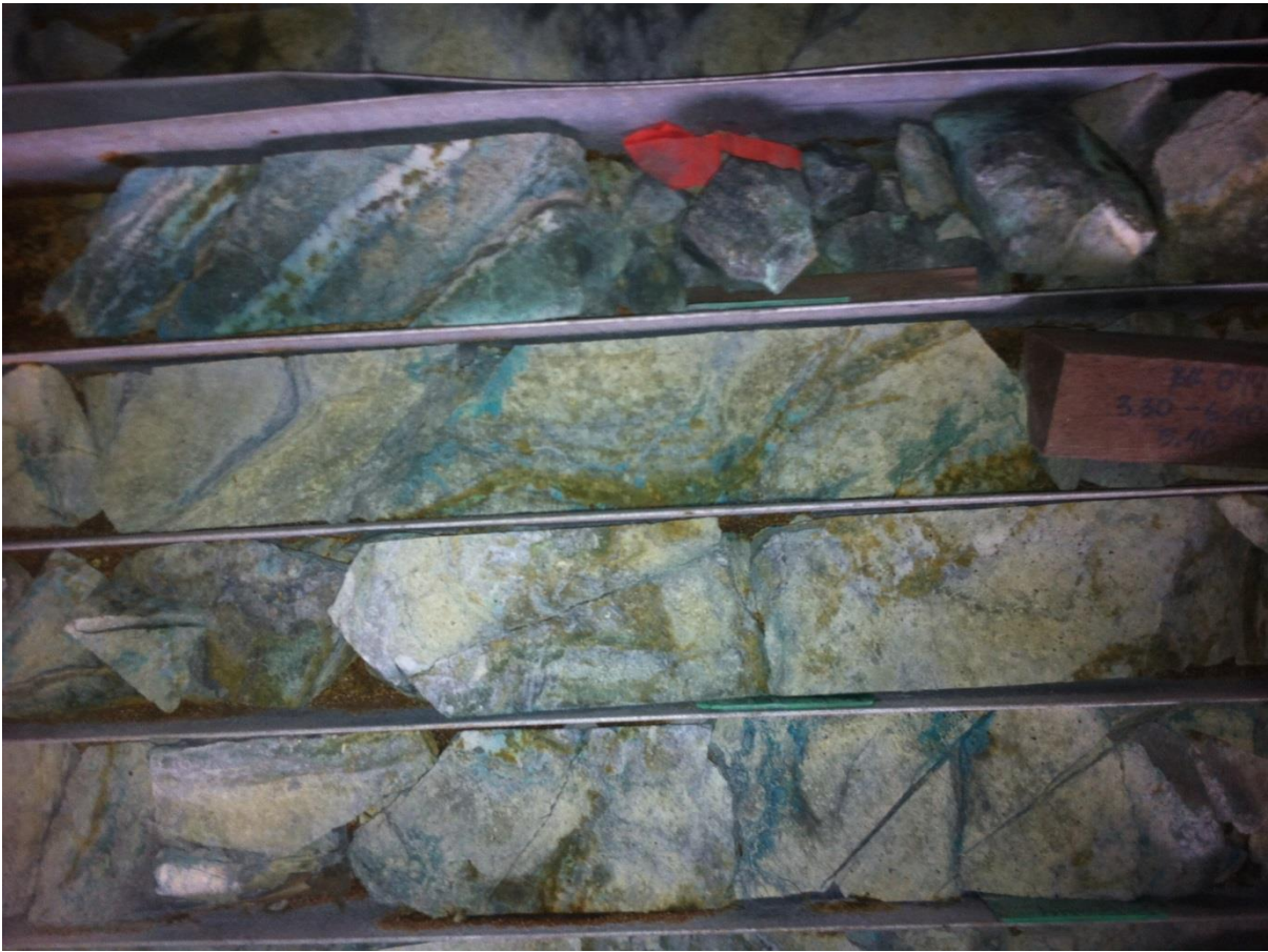
Plate 5: BK044-01, 3m – Cu mineralisation in fracture controlled pyrite veinlets and Si-Py veins. Significant secondary brochantite formed when core exposed to air.
