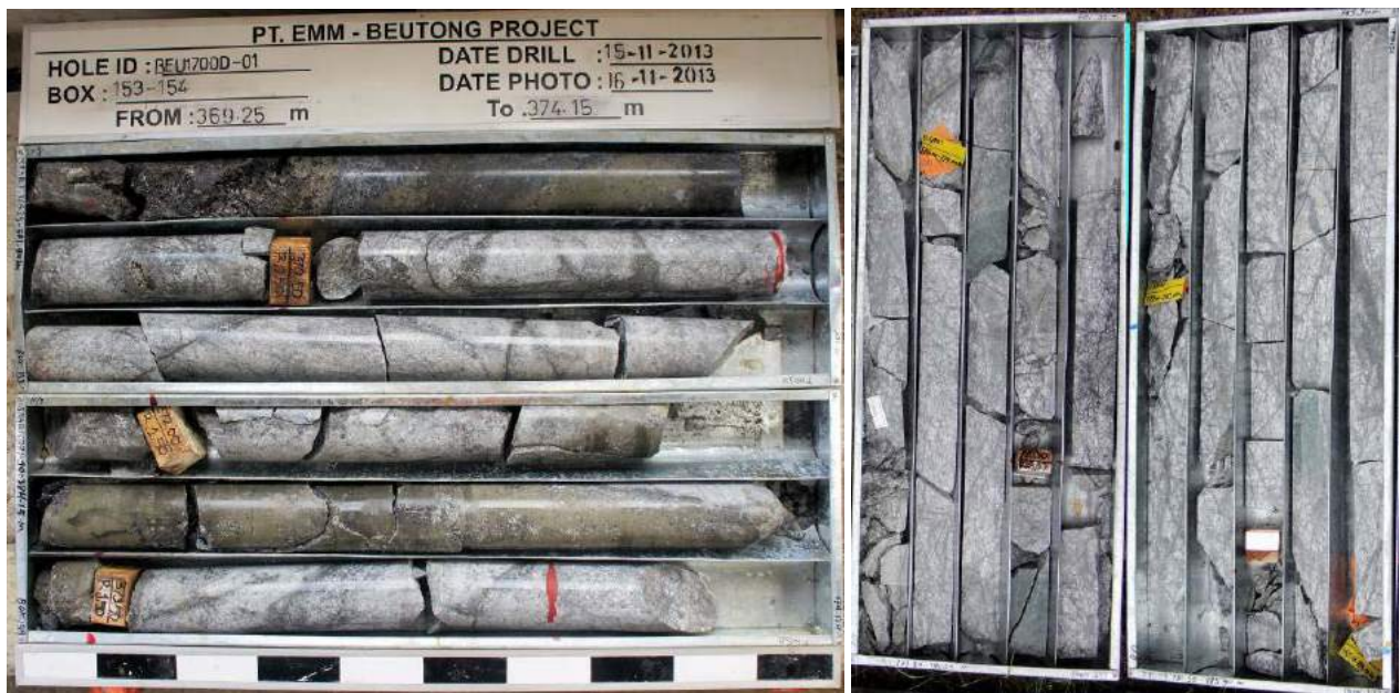
Figure 3: (Left) High sulphidation veins telescoped over the BWP (2.5m @ 7.75% Cu) (Right) Classic BWP stockwork mineralization (782 – 785m assayed 0.58% Cu and 0.34 g/t Au).
