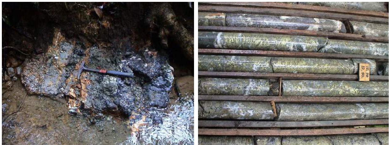
Figure 9: (Left) Outcropping Copper mineralization at Baroi Prospect. (Right) Copper mineralization in Baroi Prospect drill hole BF5.
